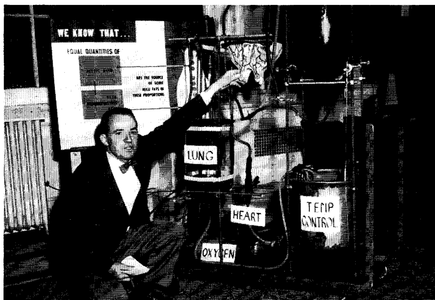
Artificial cow used for study of milk formation by use of radioactive isotopes
